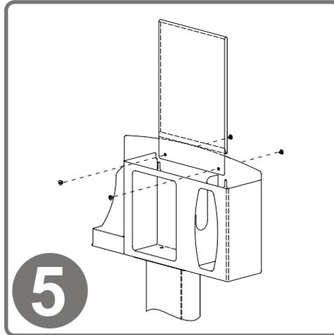
To mount the MP-070 Sign Holder, align the holes of the holder with the holes of the dispenser. With a flathead screwdriver, attach using (2x) barrel screws included with sign holder.
