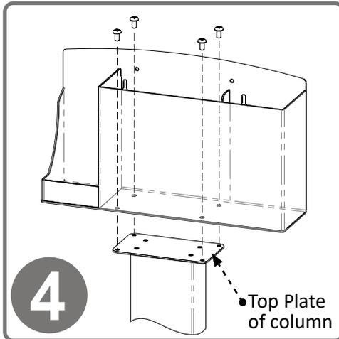
Attach the RS001-0412 Respiratory Hygiene Station to the column using (4x) screws included with stand. Tighten.
