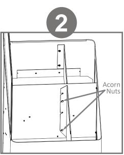
To dispense laundered gowns, loosen the four (4x) acorn nuts holding the divider in position.
