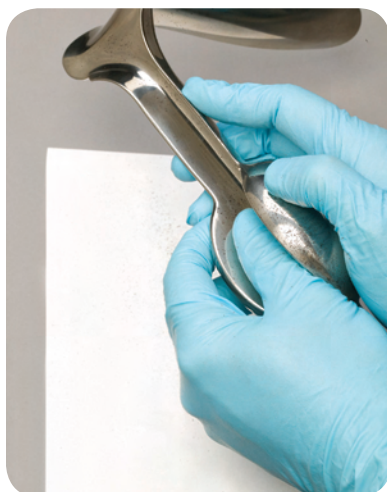
Inspect chrome-plated instruments for flaking
