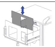
Drawer dividers can be removed by lifting them vertically from their slotted position in the drawer. To replace the divider, align it with the slots in the drawer and slide back into position.
