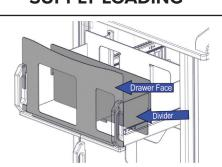
To load PPE for dispensing, open the drawer and place the supplies in the designated area between the divider and the drawer face. Verify that items are properly positioned for dispensing. When finished, close the drawer and the cart is ready to dispense supplies. Extra supplies can be placed behind the dividers.
